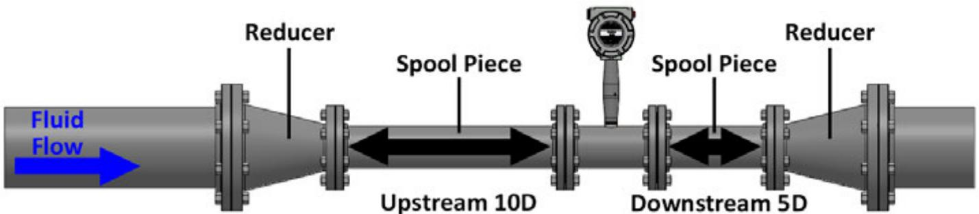
AX24R Reduced Bore Vortex with integrated reducing flanges
