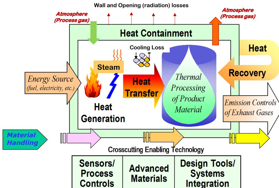
Figure 1. A fuel-based process heating system and opportunities for improvement
